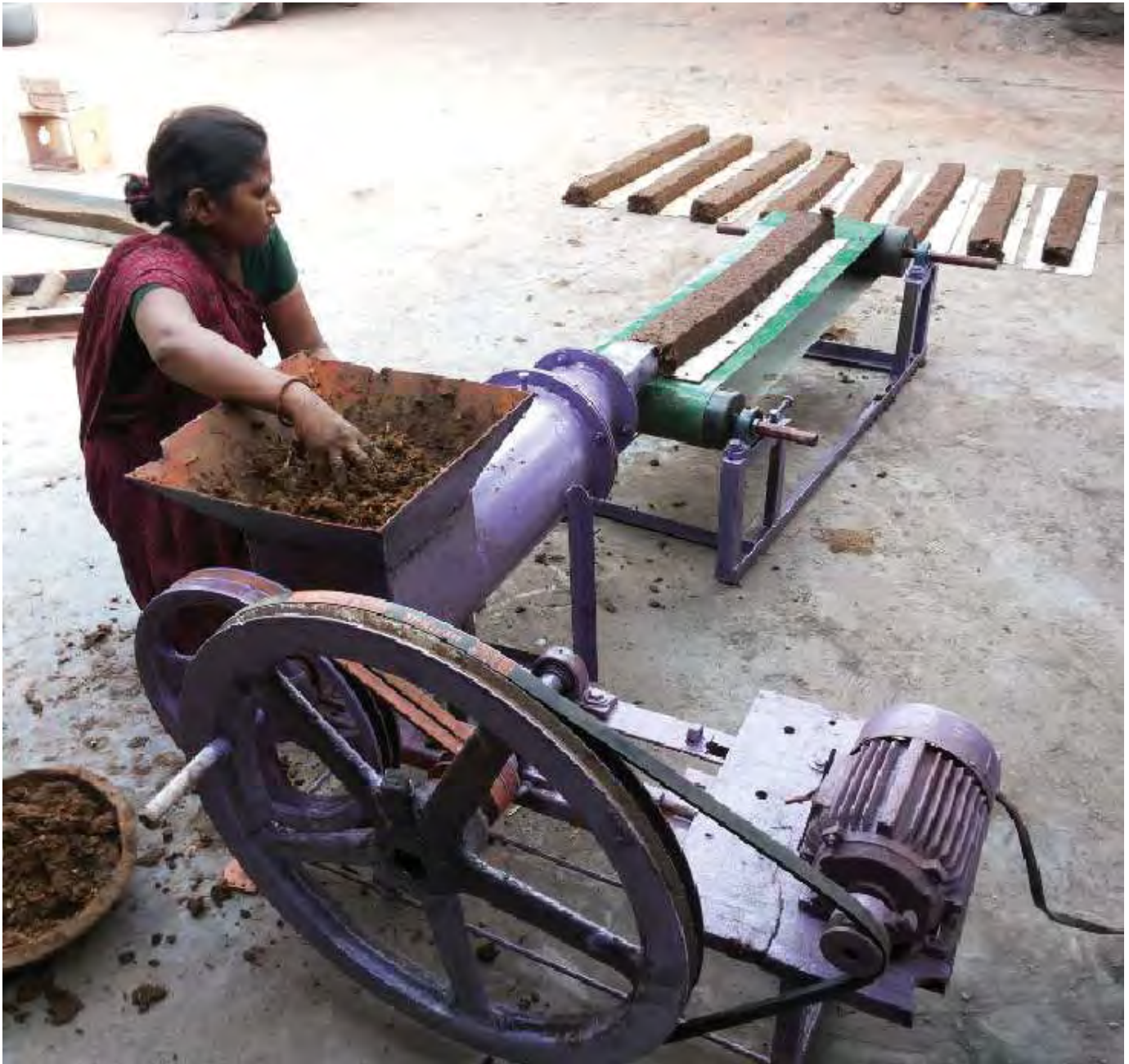
An innovative machine for making cow dung logs for eco-friendly cremation
