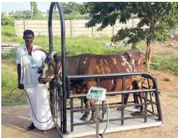
Heavy duty platform weight balance for measuring weights of animals at regular intervals to assess their health and well being
