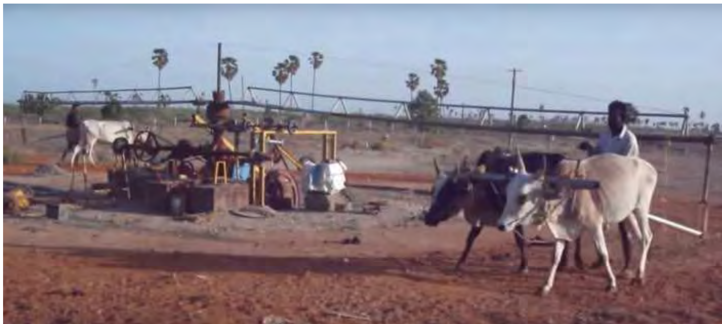
Ox Power Electricity Generator at Gorakshyam Trust managed by Gokul Ashram
