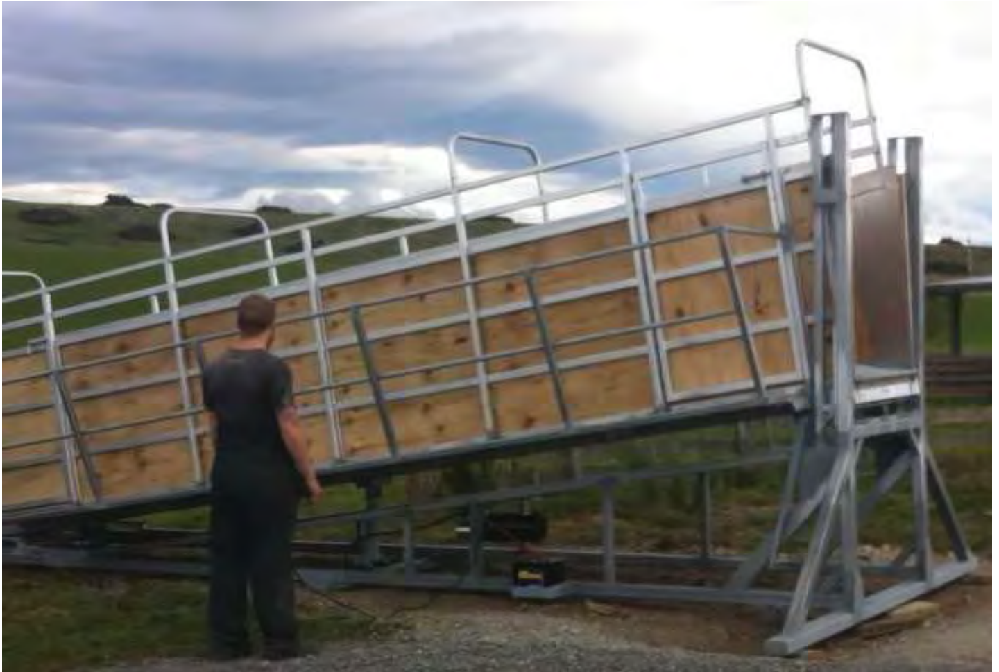
Height adjustable ramp fitted with motor compatible with all transporting vehicles of varying height
