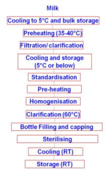
Fig. 3.3 Flow chart for preparation of sterilised milk (In-bottle sterilization)
