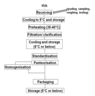
Fig. 3.2 Flow chart for preparation of pasteurized milk
