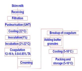
Fig. 3.5 Flow chart for preparation of butter milk
