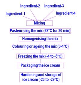
Fig. 3.7 Flow chart for preparation of ice cream
