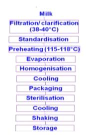
Fig. 3.11 Flow chart for preparation of evaporated milk
