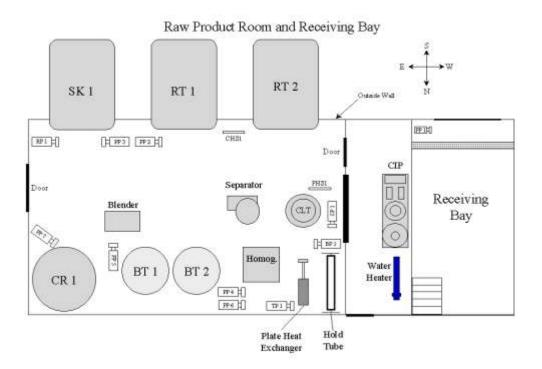
Fig. 3.16 An example of a plant layout
