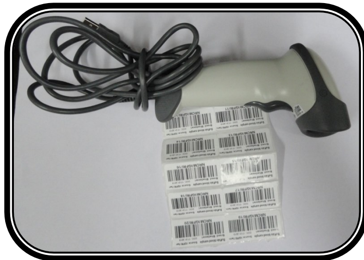
Figure 2: Bar code stickers and bar code reader
