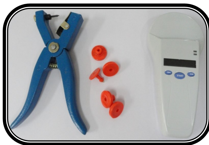
Figure 1: RFID ear Applicator, ear tags, and reader
