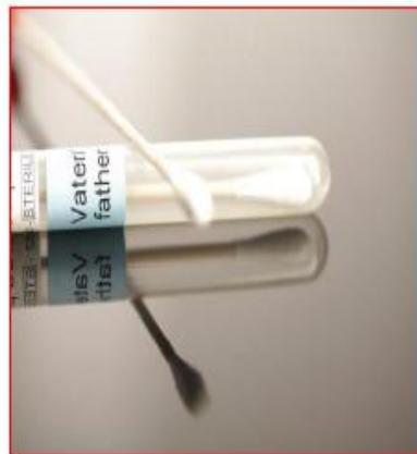
Sample soaked swabs should be inserted in sterile test tube for further examination.
