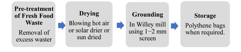
Process of fruit and vegetable waste conversion using drying method.
