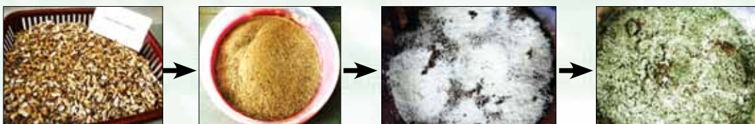
Processing of groundnut shell for production of cellulases by microbial fermentation (L-R: Groundnut shell, powdered groundnut shell; solid substrate fermentation by Phanerochaete sp. (whitish) and Trichoderma sp. (greenish))
