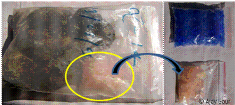
Figure 3: Scat sample and silica beads (blue turned pink) sealed in a zip lock pouch
