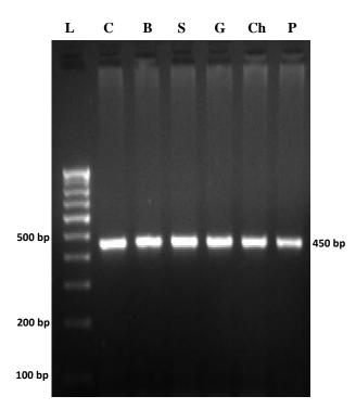
Figure 1: Polymerase chain reaction amplification of mitochondrial Cytochrome B gene of meat samples run on 1.5 % agarose gel L: 100 bp ladder; C: Cattle; B: Buffalo; S: Sheep; G: Goat; Ch: Chicken; P: Pig
