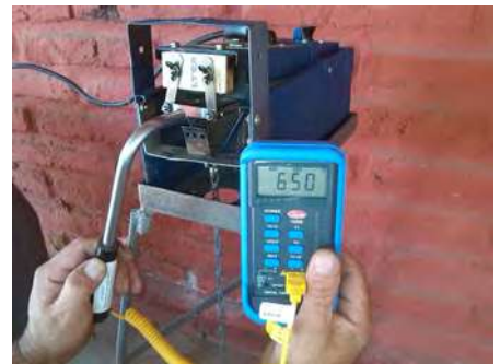
Pyrometer indicating proper blade temperature of 650°C.
