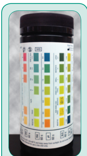
Figure 1. Multiple-test reagent strip results are compared with color scale on back of test strip bottle
