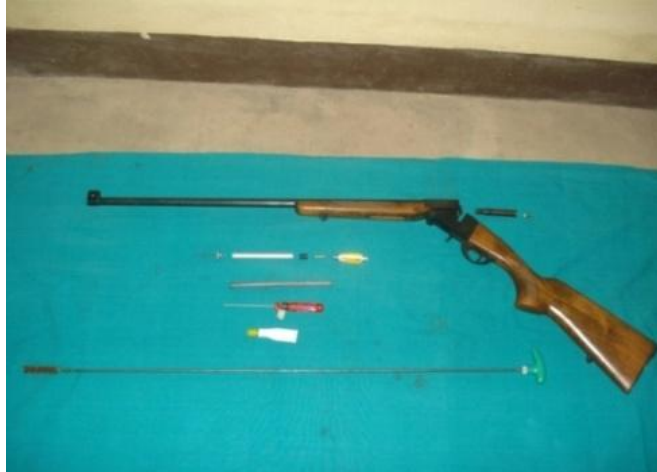
Tranquilizing gun(Syringe projector) along with accessories operated by cartridge for long range in free ranging rescue operations
