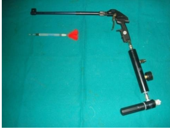
Tranquilizing gun (Syringe Projector) along with dart operated by compressed air for close range and convenient for darting small and medium animals
