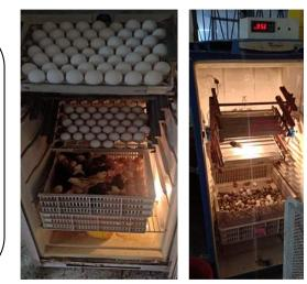
Fig. 2. Front view of Rural poultry incubator fabricated from discarded refrigerator
